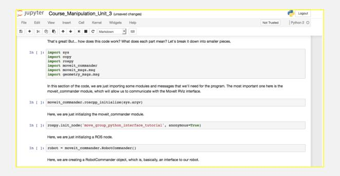
Next you add the part for approaching the object with the robotic arm. Then you make it pick up. Finally you make it lift the object. Every part can be done in a subroutine, and executed and analyzed separately.
